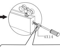
Adjust the galss parallel and 90° to floor, tight up M4\*14screw.
