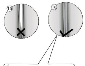
Adjust the sliding doors using the screws located on the bottom of top roller assemblies Adjust rollers so that the sliding doors are parallel to the fixed panels and parallel to each other.
