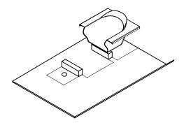
2. A )Stick a layer of protective on the surface of bathtub, and palce the bathtub in the installation position. See picture 1: Fill up two parallel lines cement bricks in the bottom of bathtub accroding to the size as picture show, to ensure the outlet is 110mm away from the ground(if customer require higher, then fill up the bathtub accroding to customer's requirement).
